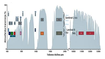
Figure 1. Spectral bands of Landsat8 and Sentinel2 [2]
