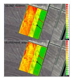
Figure 8. Results of NDVI index for RapidEye and PlanetScope
