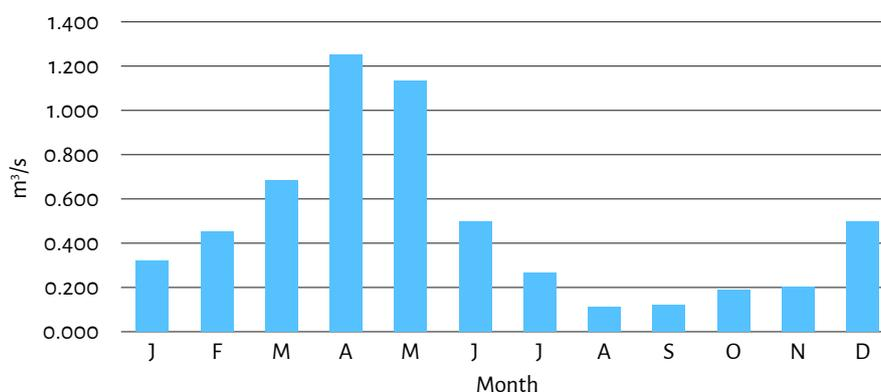
Figure 3. Hydrograph of average monthly water quantities for the period 2010–2021
