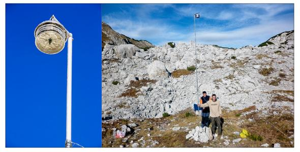
Figure 4. Measuring apparatus for the air temperature in Valoviti Do
