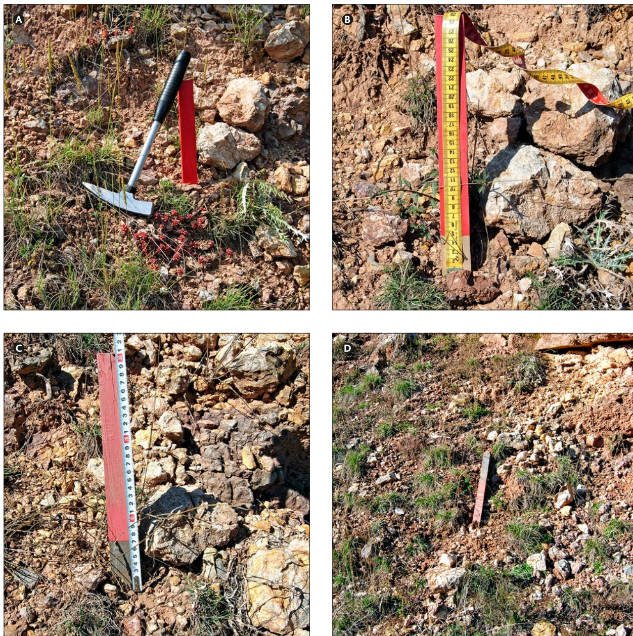
Figure 8. Regular reports on marked stake for 4- years observation period: A) time sequence - 07.07.2006 B) 29.10.2006 - 4,6 cm denudation C) 16.09.2007 - 6,6 cm denudation D) 29.11.2009 - 22 cm denudation - the rod is inverted and moved 1 m over the slope
