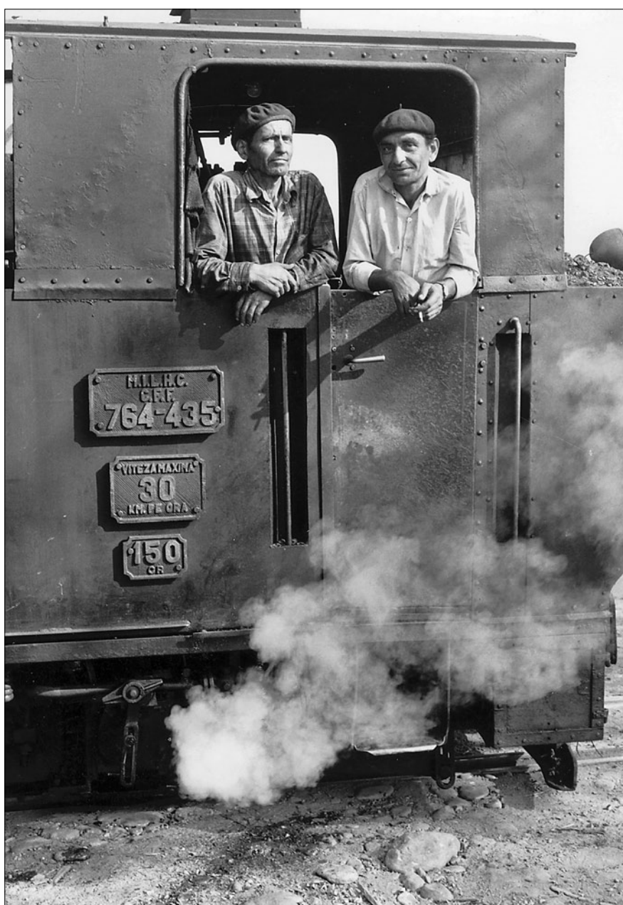
■ Plate 7 A Resita locomotive on the Tismana system (1975) with plates indicating the subordination of the CFF to the Ministry for the Wood, Paper and Cellulose Industry (MILHC), the locomotive type (76cm gauge and four driving axles - hence 764), locomotive number (435), maximum speed in km/h and horse power.
