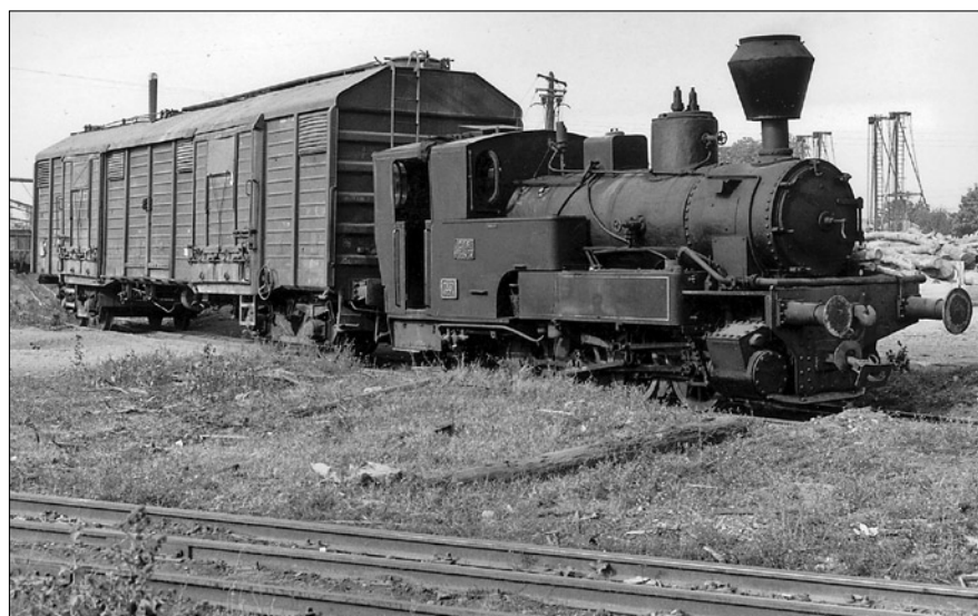
Plate 2 Mixed gauge still survives at the Orastie woodyard so it possible for a narrow gauge locomotive to shunt a standard gauge wagon (1987)
