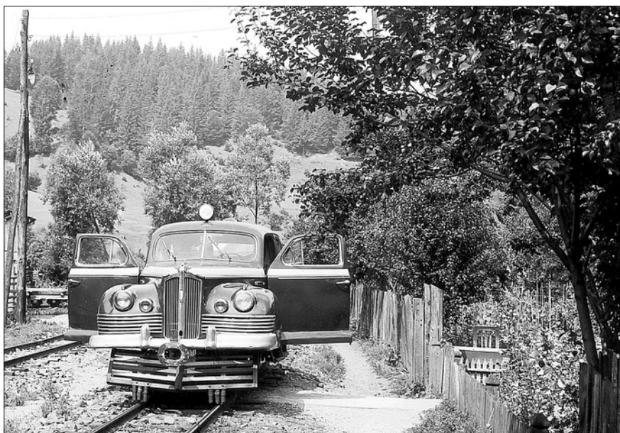
■ Plate 2 A car converted for use on the railway for management and VIP use (1977)
